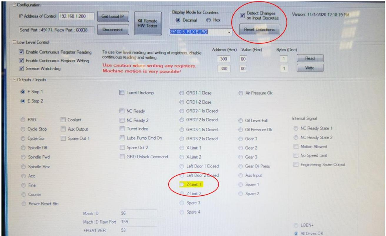
The Hardware tester can also be used to force outputs and control the spindle and axes. But this requires the outputs to be enabled and the machine to be forced into an NC Ready state:
