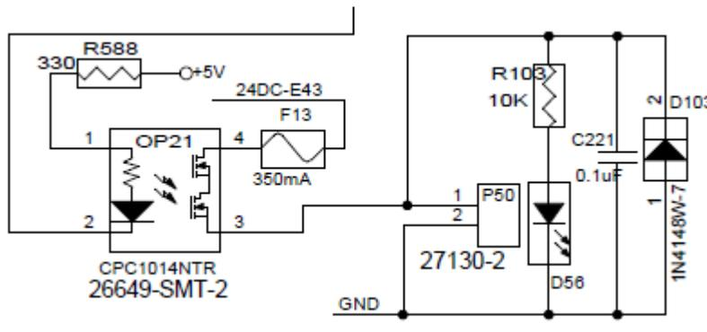
When the output is active, 24VDC will appear across the connector and the LED will be ON. Outputs are protected by self-resetting fuses, so if the LED does not come ON, check for short circuits to ground or 0V in the external circuit before considering replacing the computer module.
