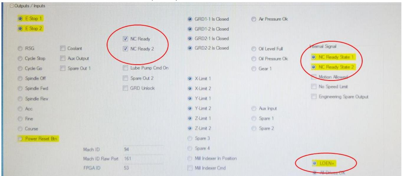
You can now turn on things like lube pumps and aux function outputs by checking the applicable box.
