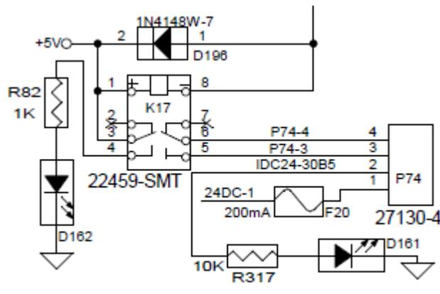
When the output is active, a low resistance (<20ohms) will appear on the output contacts and the LED will be ON. Always check the contact resistance as well as the LED, as they are on different contacts.
