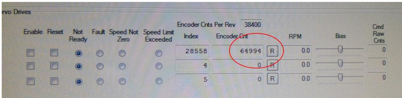
One turn of the motor is 9,600 counts (for all axes and all lathes).
