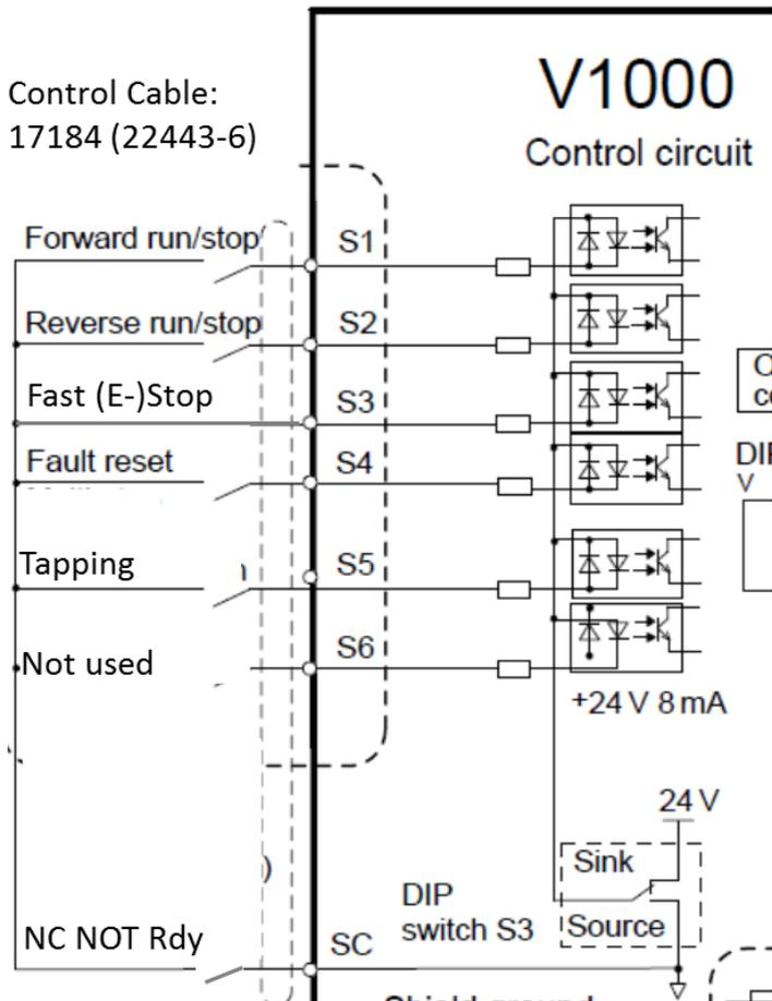
For GA500 ensure there is a link between SC and SP. Inputs S6 and S7 are not used. All other inputs are wired as for the V1000.
