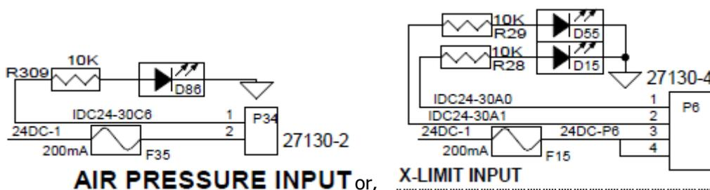
The LED is useful to indicate the state of the circuit connected to the input. When the external circuit is closed the LED will be ON. For example, if it is a limit switch input, the LED will be ON if the switch is closed (axis NOT on a limit switch) and OFF when the axis has tripped the limit switch.
